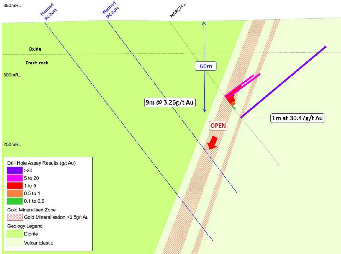
Figure 11: Cross section from previous scout drilling at artisanal mining site which returned rock chip samples up to 170g/t Au from spoil piles
