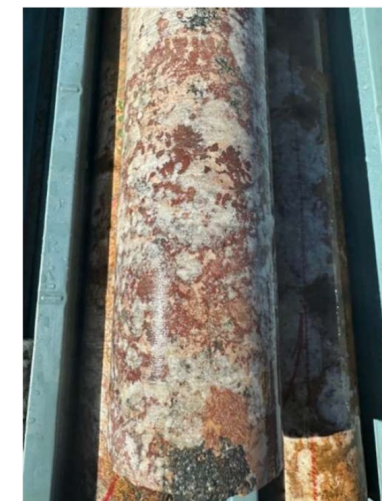
Image right: Visible rare earth mineral grains (red) in grey dolomite at 70m below surface
