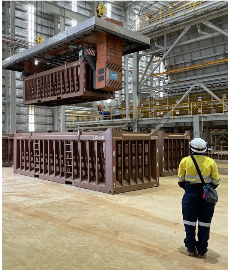
Rare earths industry first rotainer system for concentrate handling from the Mt Weld mine to Kalgoorlie
