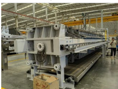
✓ Filter press built
