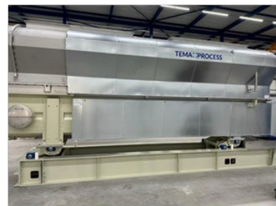
✓ Fluid bed dryer built
