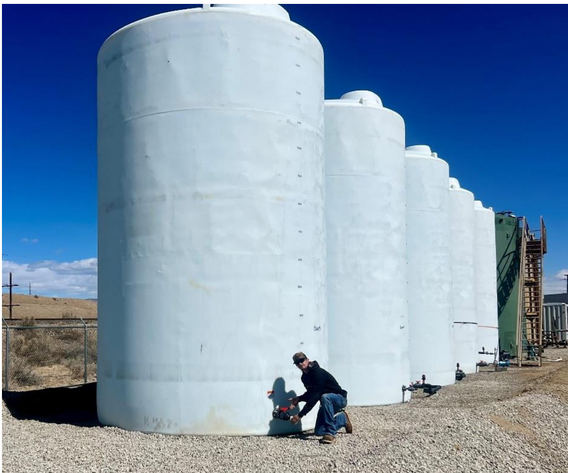
Figure 1: Photo showing the collection of sampling from the near full tanks of lithium chloride eluate produced using KTS DLE at Green River.
