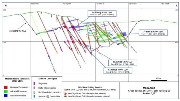
Figure 3 – Cross-section view B-B' – Main Area at depth
