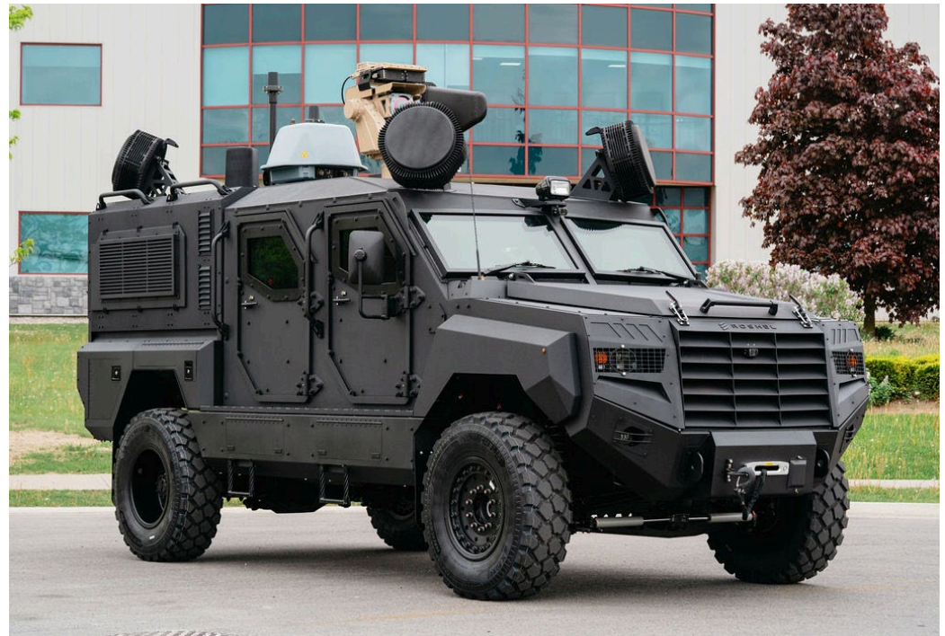
Image: Counter-UAS vehicle, featuring DroneShield's DroneSentry-X Mk2
