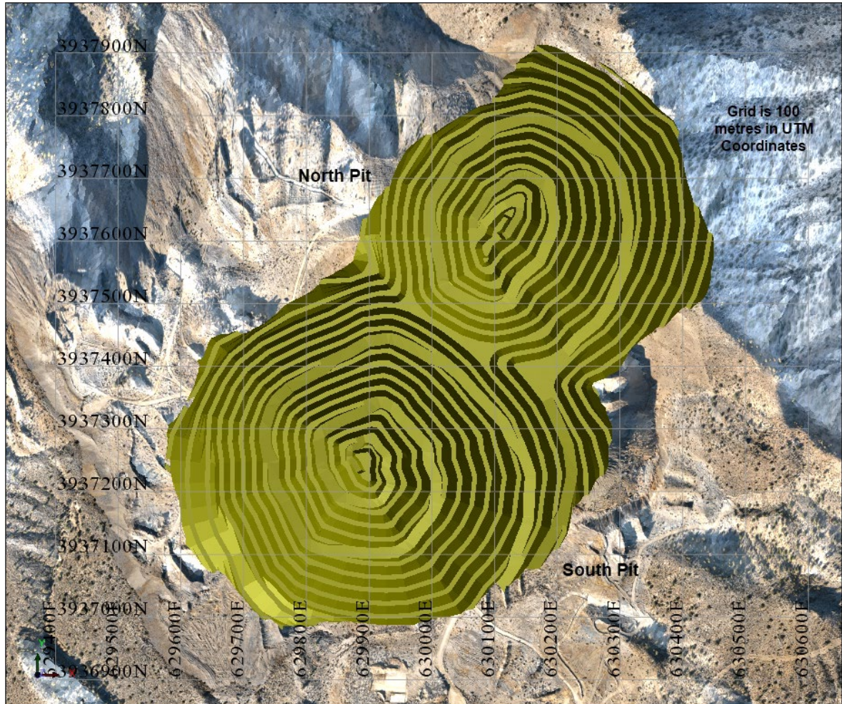
Figure 40 Final Open Pit Design
